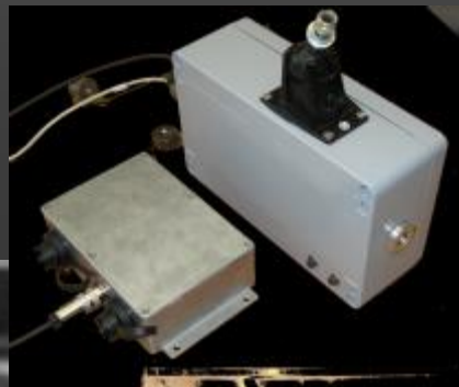
Vision analysis system to determine the presence of a tube train on a platform in order to turn off a cross-platform projector
