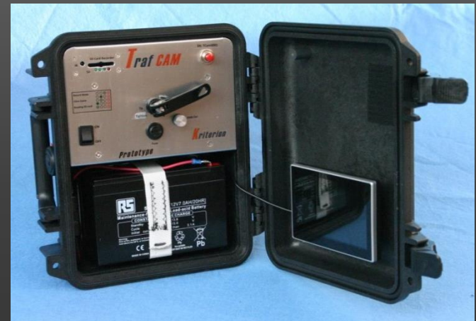
Integrated traffic monitoring camera system. Enables >24hr battery operation providing D1 digitally stored video in a ergonomically designed package.
