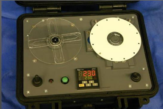
Portable mastitis field measurement kit. Integration of COTS parts into a robust measurement interrogator.
