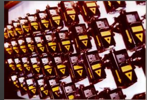
SA80 rifle mounted coded-pulse laser transmitter for use in mine clearance training applications.
